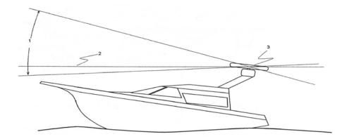
In this case, you're recommended to install the scanner so that is tilted down at the front, at an angle that will produce an almost horizontal sweep when the power boat is running at speed.
